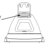
Adjust cross bar overhang to be equal both sides. Once adjusted tighten M10 crossbar bolts to 15-16 Nm (132-141 lbf.in). Then fasten M6 security screws to 3-4 Nm (26-35 lbf.in)
