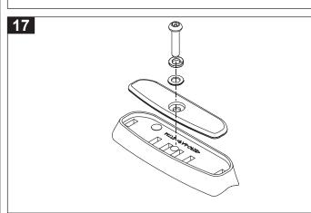
Pad cover plates are provided for when crossbars are removed.
