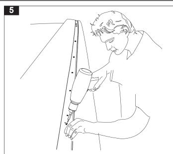
All 8 holes can now be drilled through. A drill stop must be used to prevent drilling through the hood lining on the inside. Make sure that when drilling you hold the drill perpendicular to the roof angle. The roof skin is approx. 2-3mm thick.
